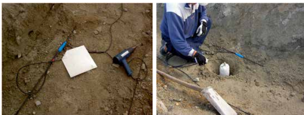
Figure 1. Installation of a) stainless steel plate electrode, b) non-polarisable electrode (Cu-CuSO 4 pre-packaged in bentonite mixture).
